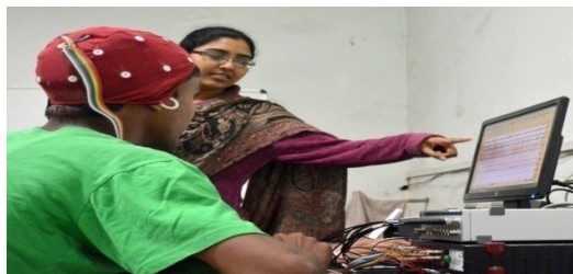
Students performing experiment to monitor various physiological signals of human body using 16 channel Biosignal data acquisition system
