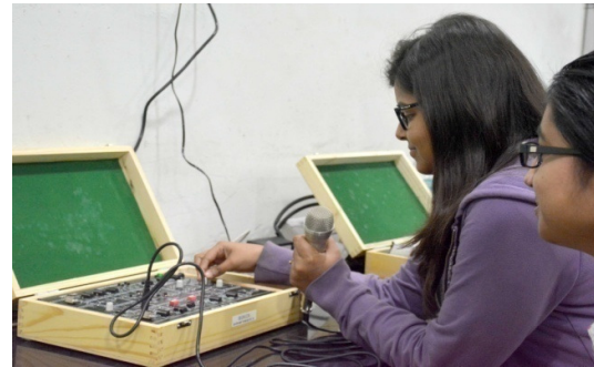
Students performing experiment to measure numerical aperture using Fiber Optics trainer kit
