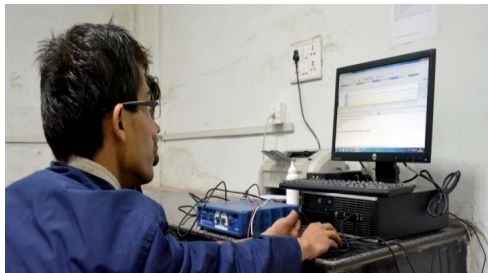
Students performing experiment to monitor various physiological signals of human body using 4 channel Biosignal data acquisition system
